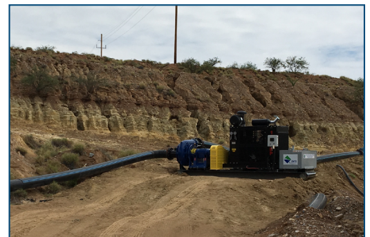
An IMS 1012 Booster Pump in operation with a 7012HP Versi-Dredge at a mine site in the United States.
