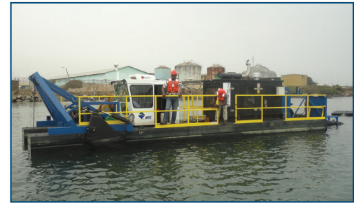
A Model 7012 HP Versi-Dredge® mines sand from a river in Monrovia, Liberia.
